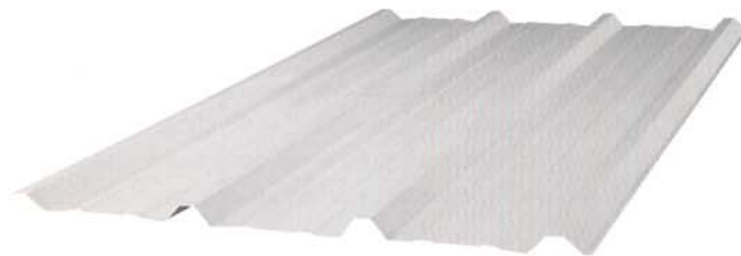
36" COVERAGE / 26 GAGE DECK AS SPECIFIED - PURLIN SPACING TO 5'-0"; JOIST SPACING 5'-6" UL90 CONSTRUCTION 176
