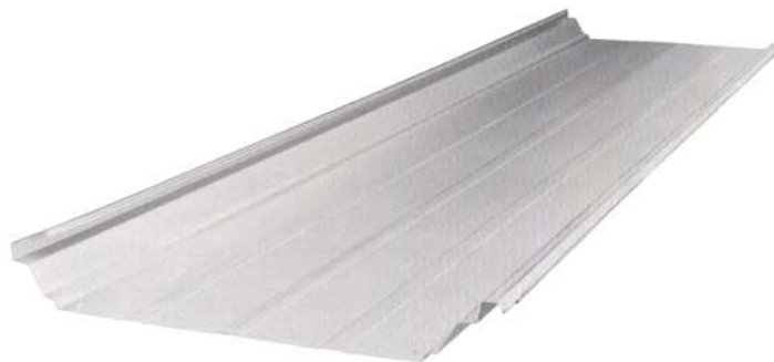
24" COVERAGE / 24 GAGE PURLIN SPACING TO 5'-0"; JOIST SPACING 5'-6" UL90 ® , FM
